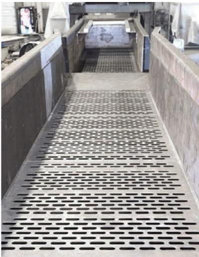
**The new machines have 1.5-in. thick steel decks stiffened to withstand impacts from 1,600-lb. steel castings, and cut with back-drafted slots to maximize sand removal and minimize product jamming.**
